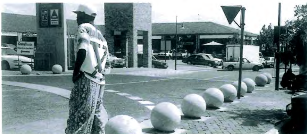
By defining the space through the use of bollards, surface material, etc, recognisable and safer pedestrian routes are created.
